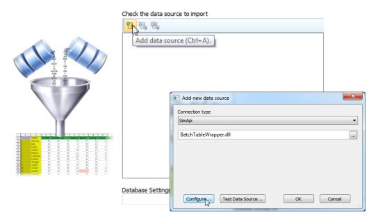
Select SimApi as connection type, find the installed BatchTableWrapper.dll and click on Configure... button and the Batch Table Wrapper Configuration is opened. Continue to 2.3 below.
